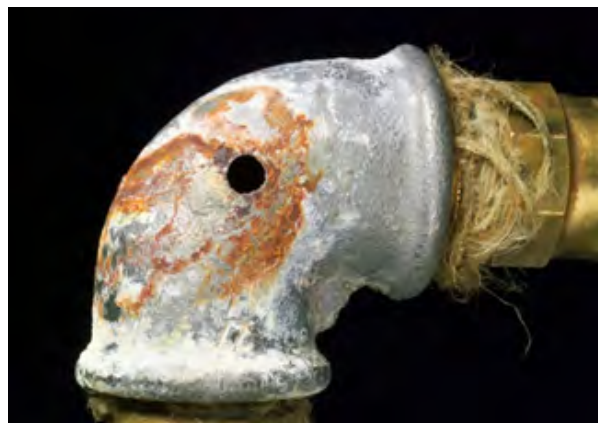
Figure 75: corrosion on pipework through the aggressive water from the sea
