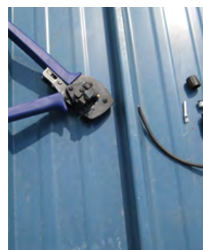
Figure 202: Prepare DC wiring within the module area and solar connector with appropriate crimping tools.
