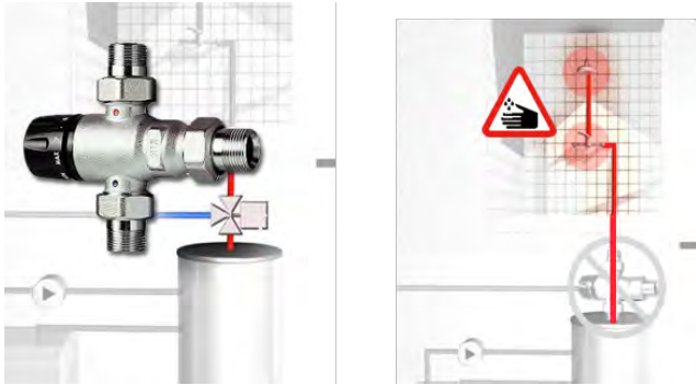
Figure 259: Thermostatic mixer should be installed in the outlet of solar system for end-user protection.
