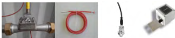
Figure 244: Flow-sensor, temperature sensor, pressure sensor an irradiation sensor (from left to right)
