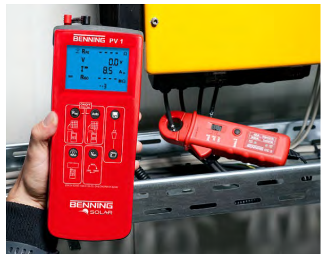
Figure 209: Solar tester to create a start-up and string protocol
